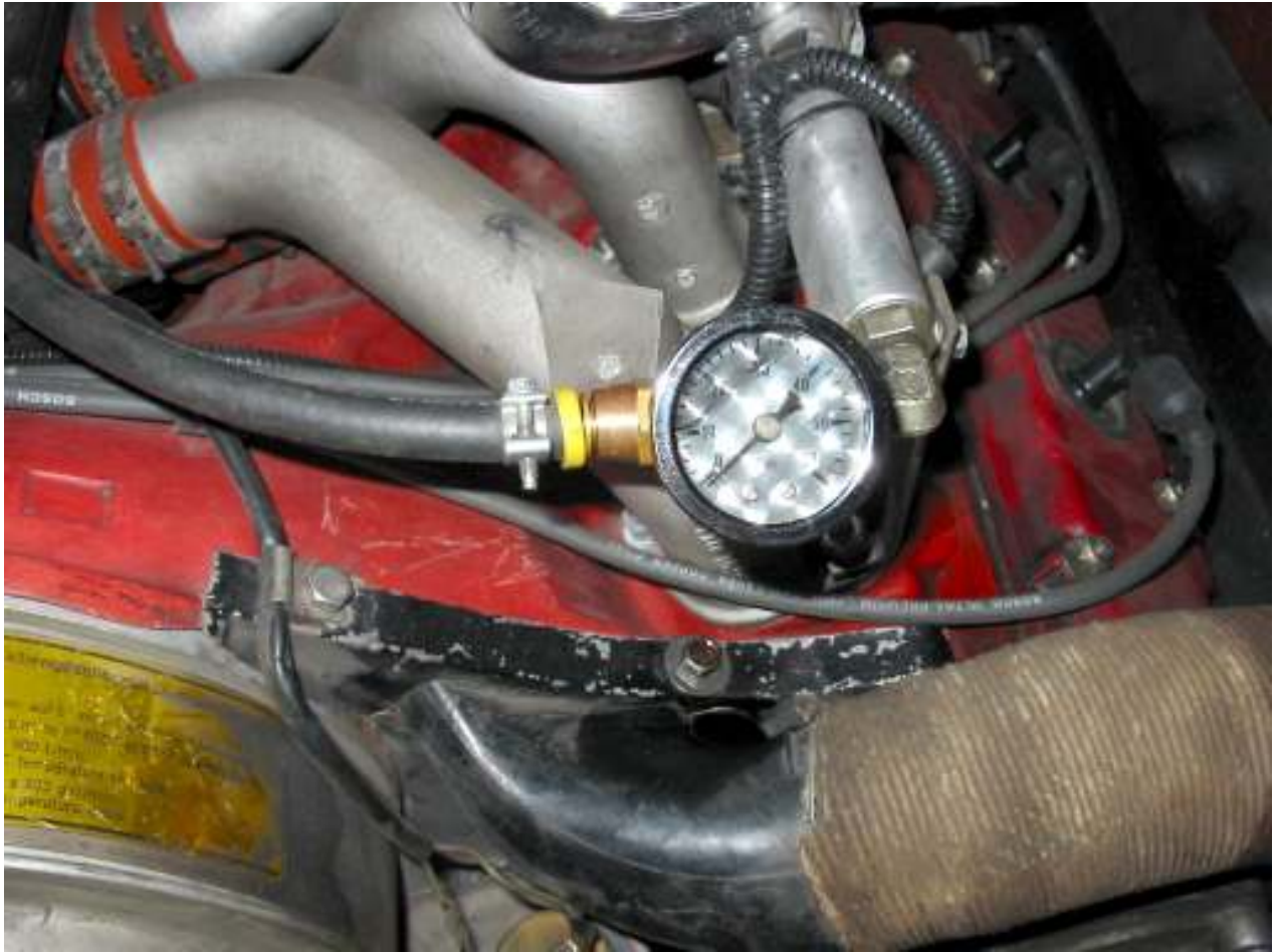
Figure 4: Gauge installed in engine bay
