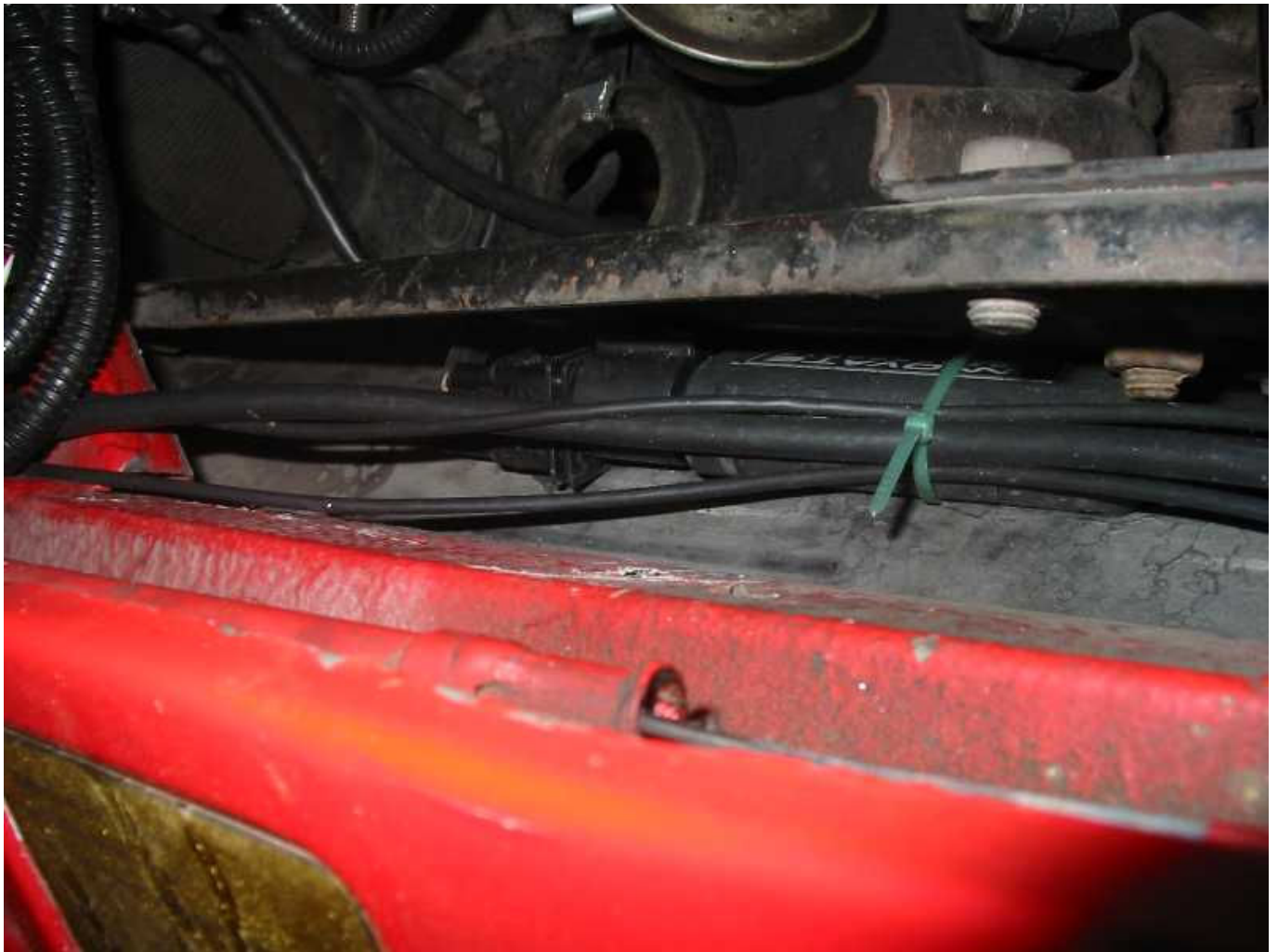
Figure 5: LC-1 mounting location
